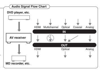
If signals are present at more than one input, the inputs will be selected automatically in the following order of priority: HDMI, digital, analog (including multichannel). You can specify which audio inputs the AV receiver checks for the presence of a signal in the "Automatic Audio Input Selection Setup" on page 47.
